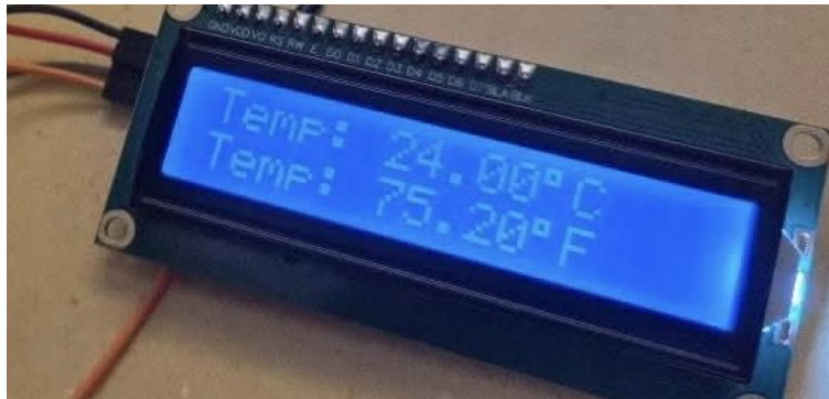
Figure #4: This Figure shows the LCD displaying the temperature recorded from the DS18B20 temperature sensor in both Celsius and Fahrenheit.
